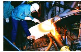
With Hotwork service, the sintered glass can be deposited at a position where the factory can most conveniently handle it for further use as cullet. The photograph on the brochure cover shows glass being deposited in a yard outside of the furnace building, from where the factory could transport it to their cullet storage facilities, using mechanical shovels and trucks. Other possibilities exist, of course, and frequently the cullet is deposited in a designated cullet bay.
