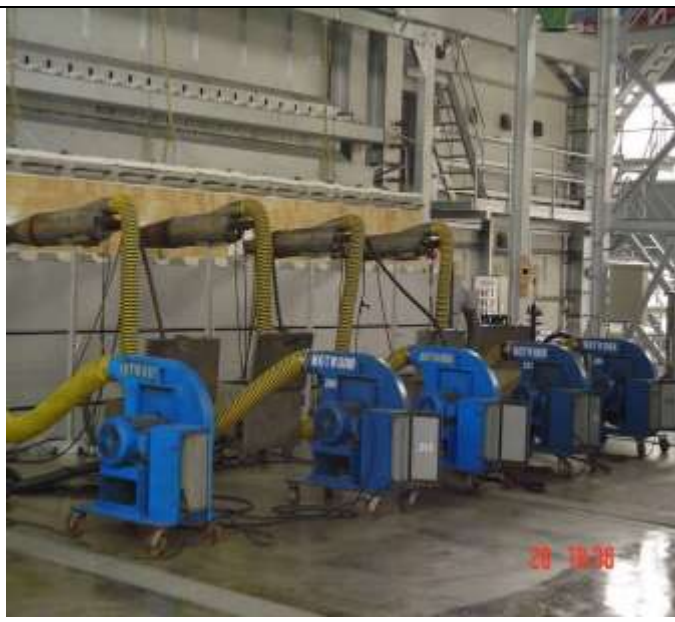
Figure 23: Float Glass Furnace heatup.
