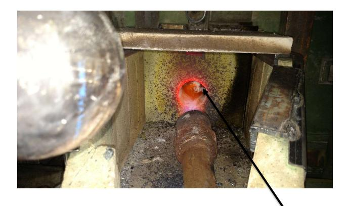
Remains of the fiber balls, used to heat up the drain hole overnight. Cold glass still in the hole, being heated by a burner.
