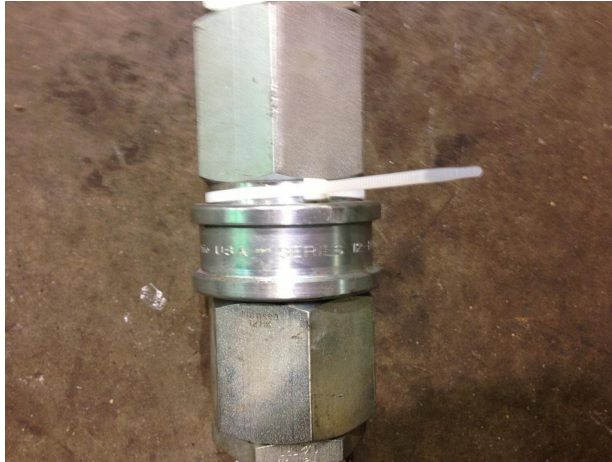
Zip tie to prevent inadvertent sleeve retraction.
