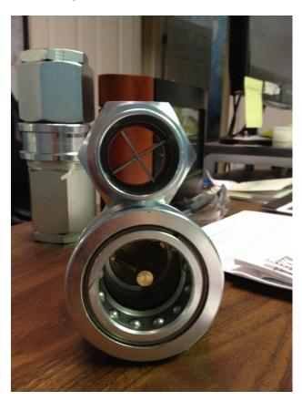
These fittings operate similar to the oil fittings where an outside collar must slide forward to lock the fitting closed. The fitting is designed such that if the collar is forward, the fitting is locked. When the collar goes forward, there is a distinctive click.
