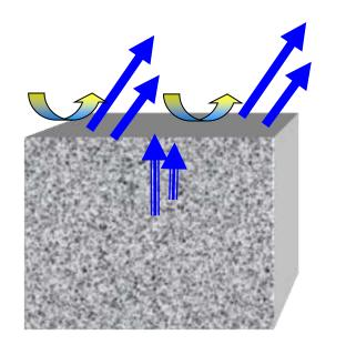
As heat is introduced during the early stages of dryout, moisture is pulled up towards the surface.
