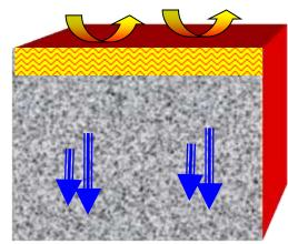
When the surface temperature reaches the boiling point, moisture is pushed by vapor pressure to the cooler areas
