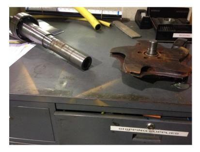
Here's a closer view of the threads on the impeller. The threads had been completely stripped for most of the shaft length.
