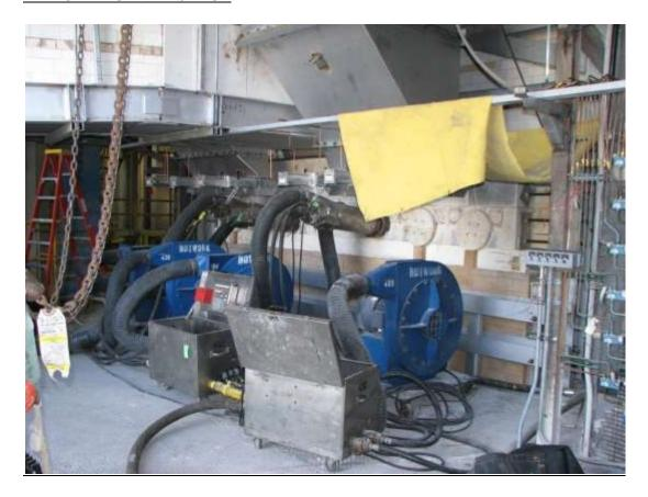
This is a photo of a standard set of heatup equipment and the number of burners used is dependent on the size and complexity of the furnace. This shows the burner, combustion air fan, and fuel train with all of the safety gear inside.
