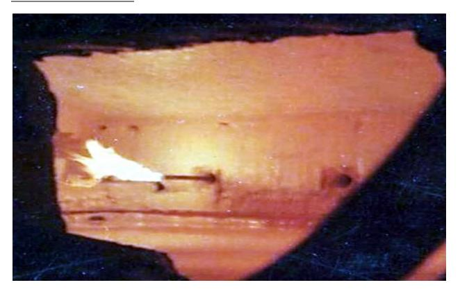
This is a photo of a gas pipe or stick burner as they were called that was provided by Mr. Phil Ross on one of the last glass furnace heatups that he did before the introduction of our technology. Many of these pipe burners were used on even small furnaces in an attempt to eliminate hot spots near and above the burner flame.
