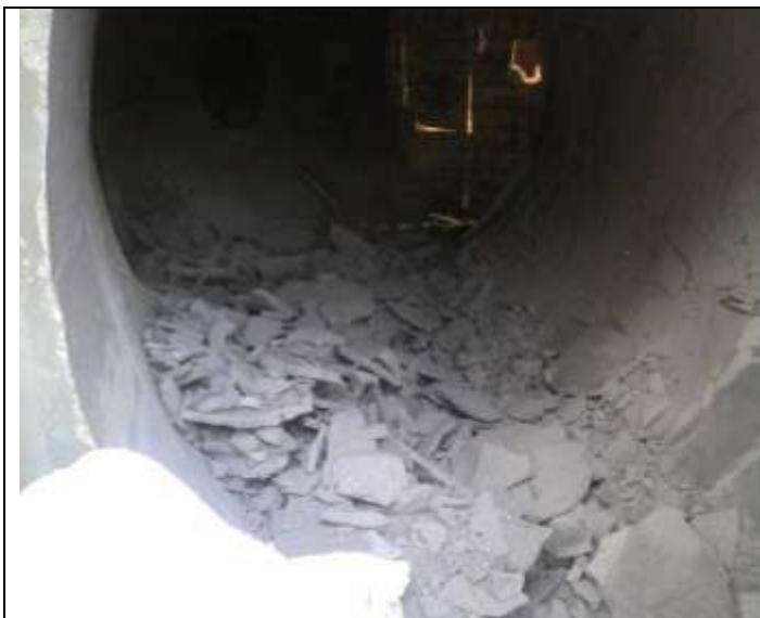
Figure 13: Explosive spall in a refractory lined duct.
