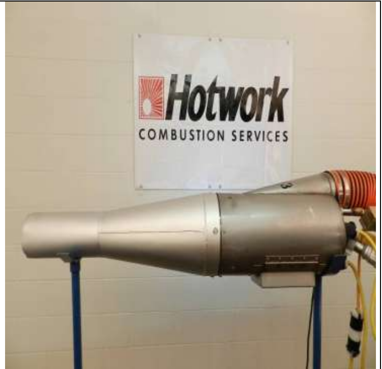
Figure 2: 10M BTU / hr High Velocity Burner
