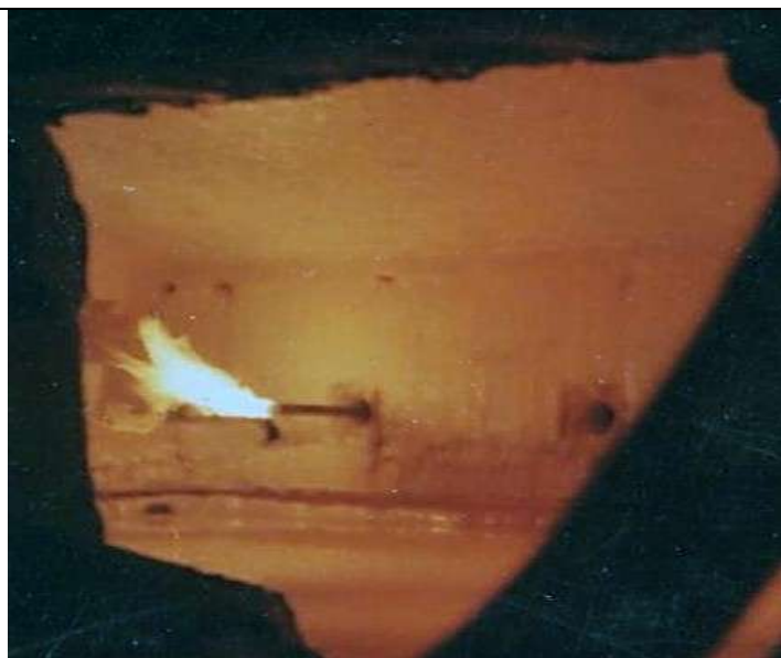
Figure 10: Typical pipe burners used for glass melting furnace heatup pre Hotwork 1962.
