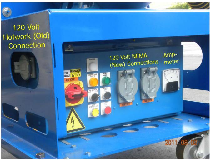
New Hotwork blower control box. Note different electrical connections:
