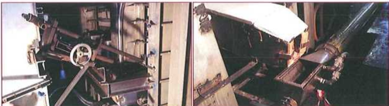
Supporting steel drill frame removed giving an obstruction free pathway to the tapping point and location
