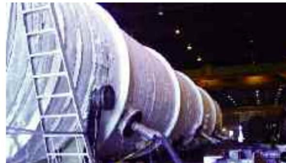
Hotwork has successfully performed Post Weld Heat Treating on vessels of virtually every size and shape in shop and field. Due to tight tolerances and temperature uniformity requirements, our combustion systems and skilled field crews are ideally suited for these projects. Since the early 1970's Hotwork has stress relieved hundreds of vessels worldwide. Our field crews are supported by managers that are specialist in this field. We comply with ASME Section VIII, BS 5500, and AS 1210 codes.
