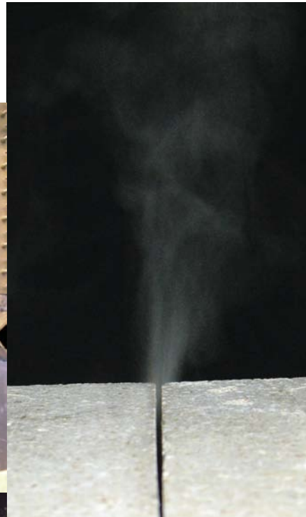
Hotwork does not extend temperature "hold" times for low pressure steam visible at the furnace shell. The steam that damages refractory is internal, invisible high pressure steam.
