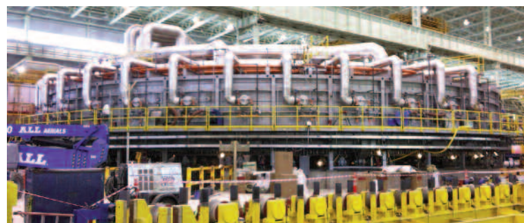
Hotwork burners at work at a rotary hearth furnace
