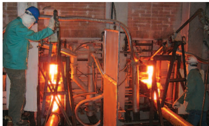
Right, left and above: Glass furnace drain and heatup
