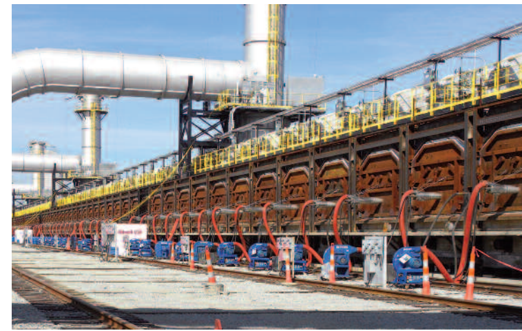
Heat recovery coke battery start up
